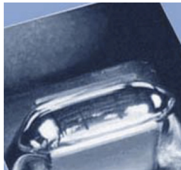
Fig. 2 Typical selective solder fountain for re-work
