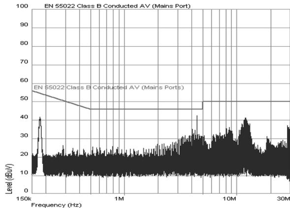
Figure 3 - Example of Class B filter response, from DC/DC converter technical specification
