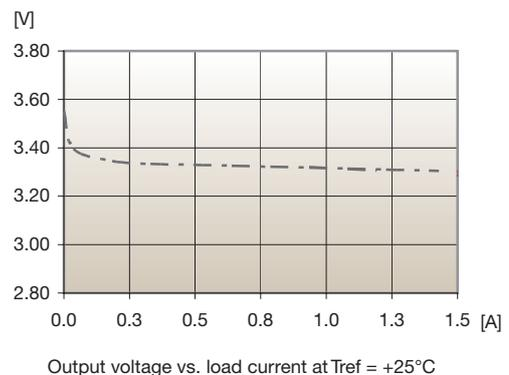
Figure 5 - Example of load regulation for DC/DC converter with diode rectification
