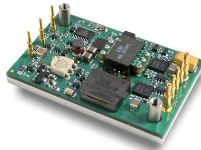
Figure 1 - Example of DC/DC converter
