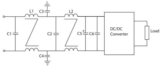
Figure 2 - Example of EMC filter design, from DC/DC converter technical specification
