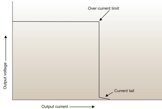
Figure 11 - Example of Over Current Protection with constant current limiting
