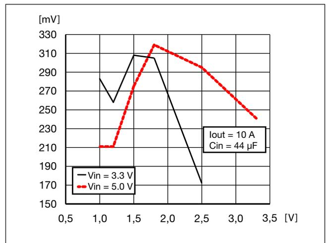
Figure 6 - Input Ripple Voltage vs. Vout - PMC4518.
