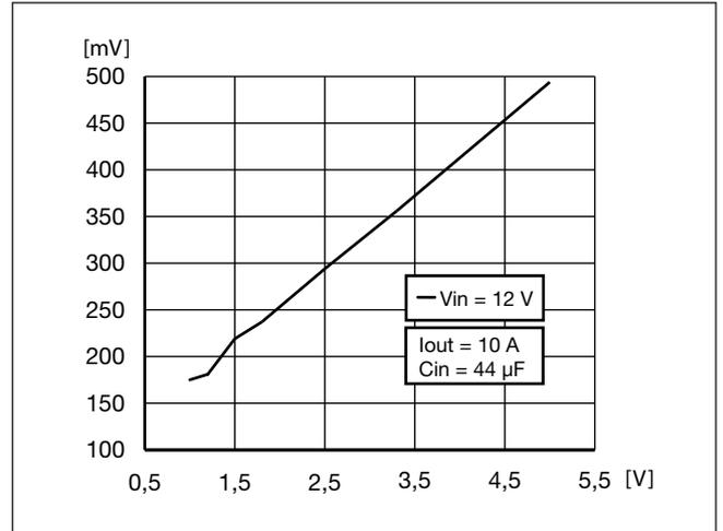
Figure 8 - Input Ripple Voltage vs. Vout - PMB8818.
