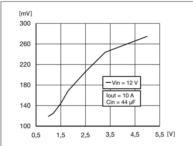
Figure 7 - Input Ripple Voltage vs. Vout - PMB8518.
