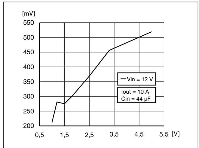
Figure 10 - Input Ripple Voltage vs. Vout - PMC8818.
