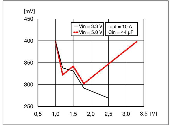
Figure 4 - Input Ripple Voltage vs. Vout - PMB4518.
