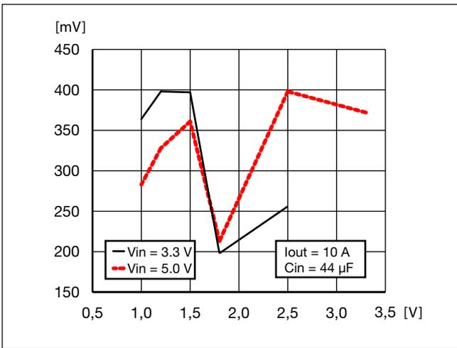
Figure 5 - Input Ripple Voltage vs. Vout - PMC4418.
