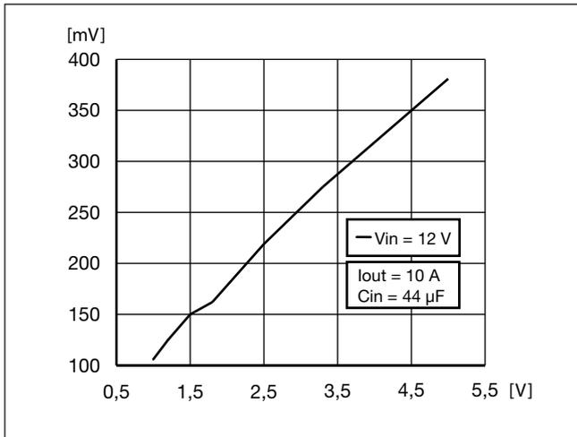
Figure 9 - Input Ripple Voltage vs. Vout - PMC4518.
