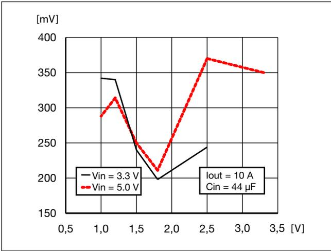
Figure 3 - Input Ripple Voltage vs. Vout - PMB4418.
