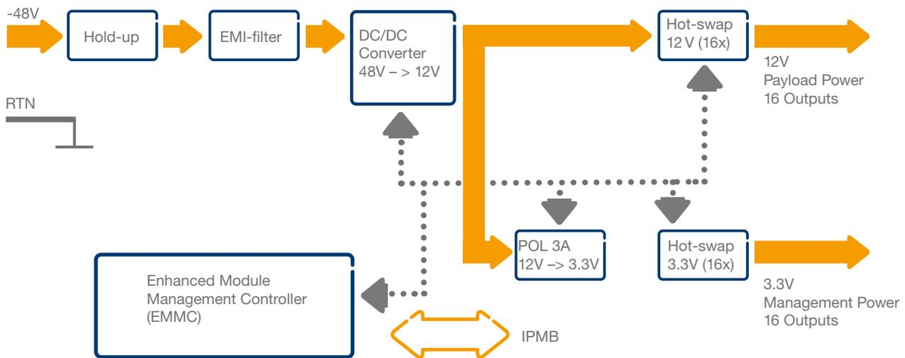
Figure 2 - MicroTCA power module block diagram
