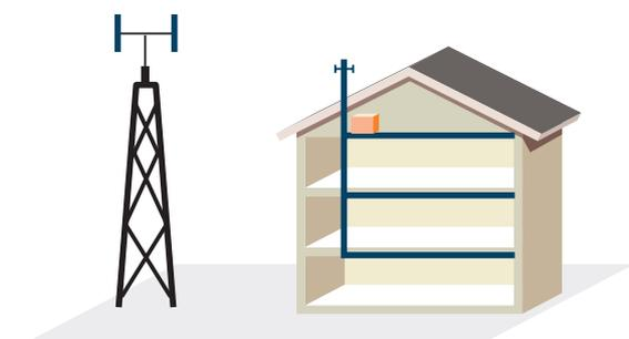
*Repeater used to provide in-building coverage from a surrounding macro cell.*
